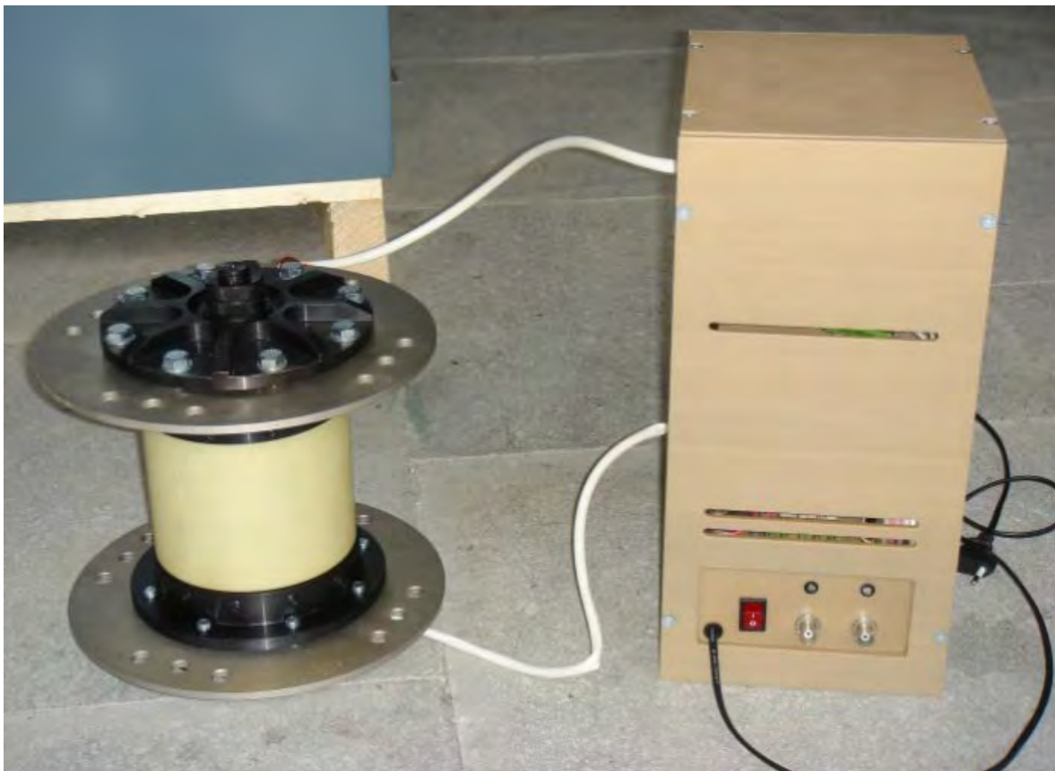
Fig.10. RSD commutator 300 kA, 25 kV DC with control generator
